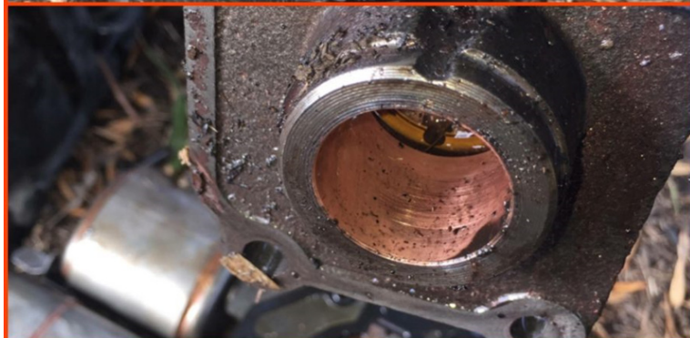
Copper plating on a bearing journal due to acids formed by moisture left in the system. A victim of improper evacuation.
